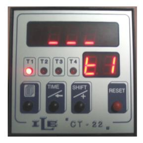
Write the password with the keys TIME/SHIFT/RESET. If this is introduced corrected the tool goes to the down-counter mode, with the desired working shift .
