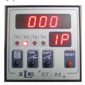
In these pages (it appears for each shift ) the foreman is able (using the keys TIME/SHIFT/RESET) to input the passwords for the entry in every shift .
