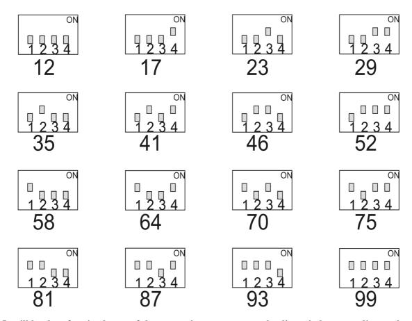
It will be therefore in charge of the system integrator to set the dip-switches according to the speed limit.
